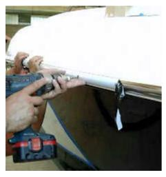
To fix the stainless steel strakes, we recommend that you start from the bow, slightly bend a bar (strakes) in the middle, so that on board itself on the right and left it creates the same lengths.
