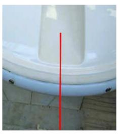
For technical reasons, it is imperative that there is no hole in the centre of the bow curve, or in the centre of the edges at the stern.
