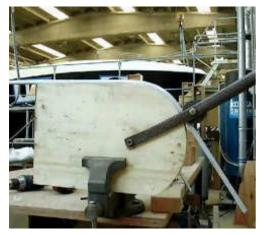
Tessilmare offers a bending service where, for a fee, you can get readycut units for bow and stern with radii smaller than 40 cm. Alternatively, you can also make horizontal and vertical bends yourself with bending disks, which perform the same function.
