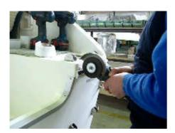
We recommend the professional use of special discs designed for stainless steel, or flex tools, for cutting to length.
