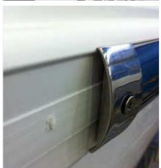
Please note that, if possible, no drill should come into contact with the stainless steel parts, because often iron drills can superficially damage the stainless steel and thus rust can form. We therefore also recommend that you seal the hole with silicone or Sikaflex, as this seals and insulates, as well as making the screw connection soft against the hull.
