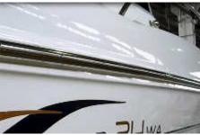
Wherever there is a joint between the profiles, a cover cap should be placed to cover the joint.
